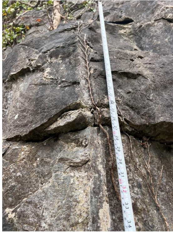
Photograph 6 – Leftover mark (where the ivy stem is growing) of a 2” drill hole that may have been drilled to install explosive (probably blasting gelatin otherwise known as “gelignite”) for blasting the rock.
